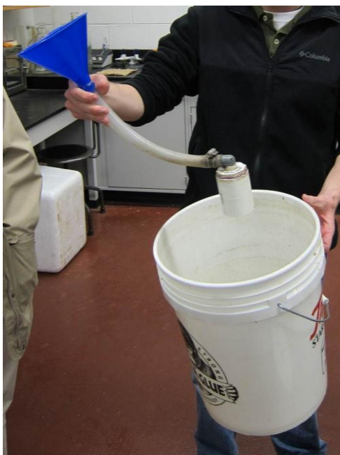
Figure 3- 2. Effluent screen set up.
